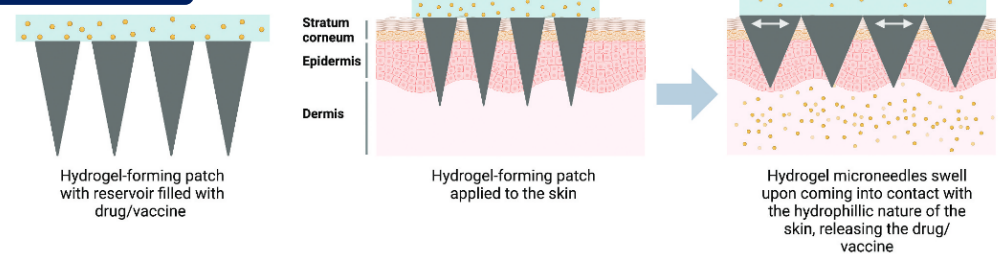
Figure 5. Schematic representation of the hydrogel-forming MAP. hydrogel-forming MAPs are fabricated with polymers crosslinked with gelatin which rapidly swells upon penetration into the skin and eventually releases the drug/vaccines into the microenvironment. Created with BioRender.com.
